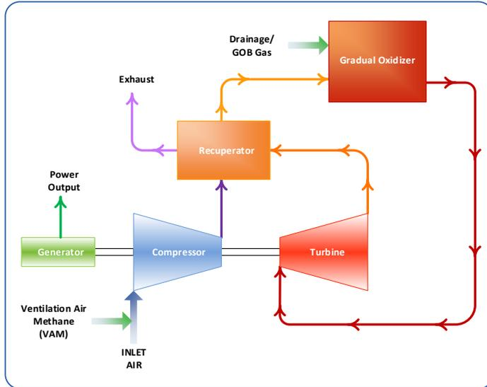
The process flow for this "dual" configuration is shown in the figure on the left. A dual-feed approach is utilized because the VAM alone doesn't contain enough energy to operate the Powerstation. During operation the Powerstation will control the amount of GOB gas injected in the oxidizer to regulate the energy input. As the VAM concentration fluctuates, the GOB gas flow rate will be increased or decreased to maintain the gas energy conditions in the Gradual Oxidizer.
